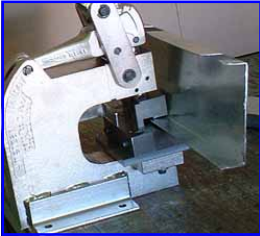
Steel Construction Studs being notched
